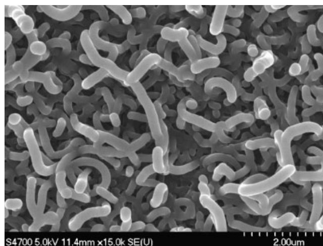
Figure 2 Scanning electron microscope (SEM) image of bent carbon nanotubes.
